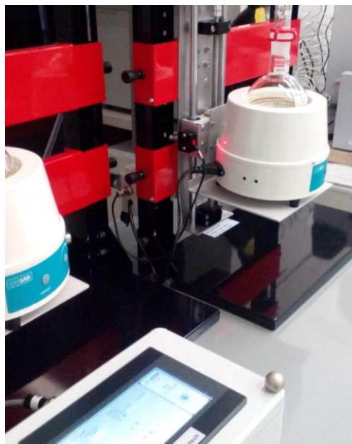
Details of automated vertical lift and heating mantle of an EIM - PADS ®
